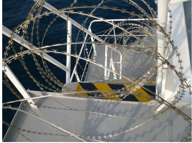
RAZOR WIRES INSTALLED AT STAIRCASE AS PART OF ANTI-PIRACY MEASURES
